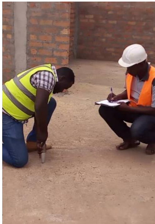
Photo plate 08: Rebound hammer tests for compressive strength on concrete members
